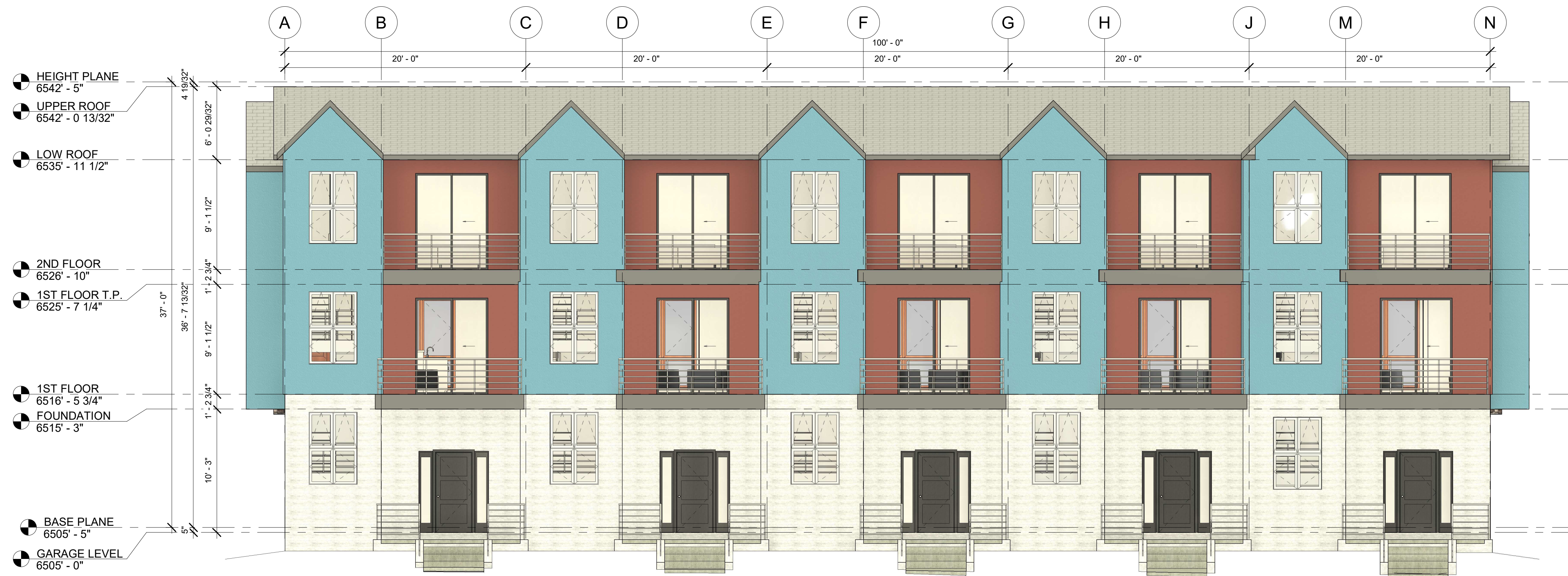
2 EAST ELEVATION (FRONT ENTRY) 3/16" = 1'-0"
