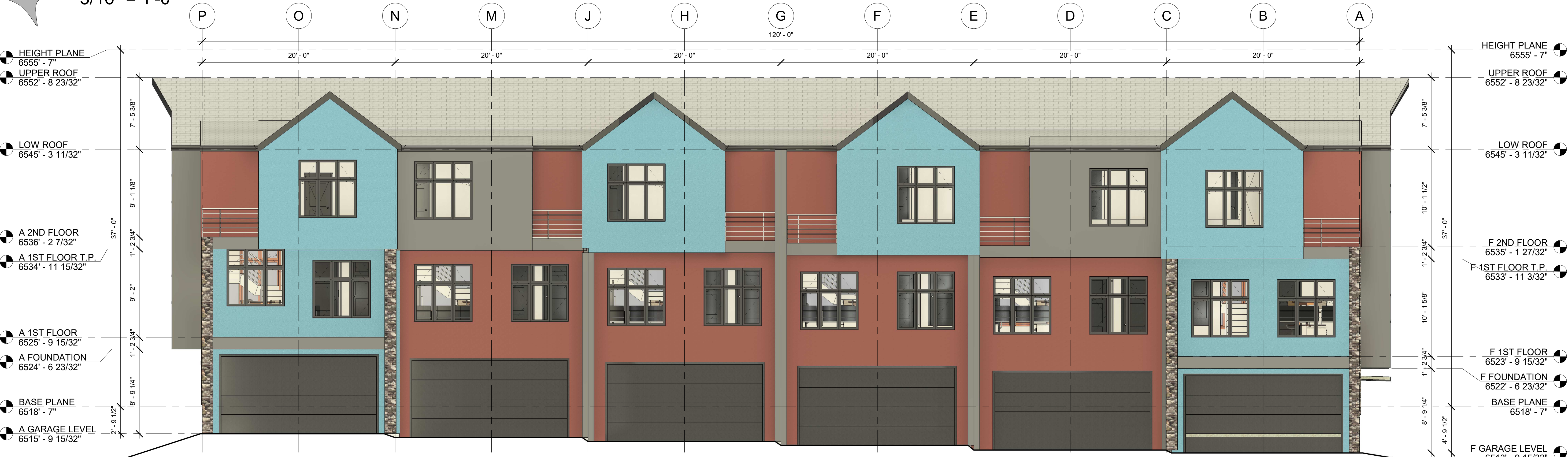
2 EAST ELEVATION (GARAGE ENTRY) 3/16" = 1'-0"
